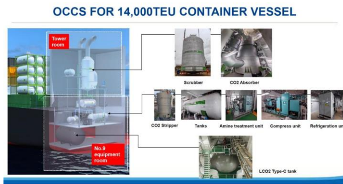
Figure 27. Overview of SMDERI-QET’s OCCS system onboard the Ever Top
