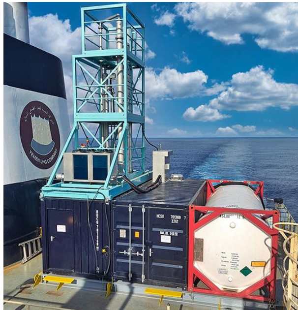
Figure 38. EverLoNG Onboard Carbon Capture System
