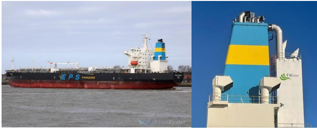
Figure 13. The PACIFIC COBALT (9788617) and OCC system from Value Maritime Filtree
