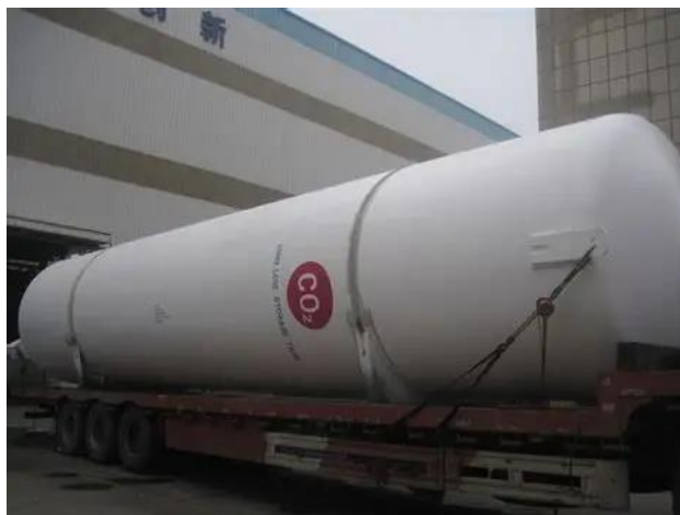
Figure 8. Liquefied CO 2 storage tank (Source: BI-Cryo)
