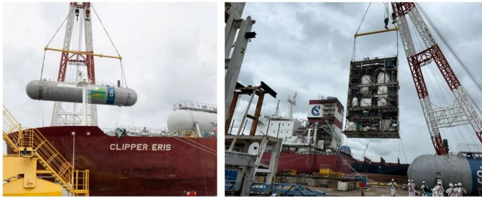
Figure 28. Installation of CCS onboard Clipper Eris in Singapore
