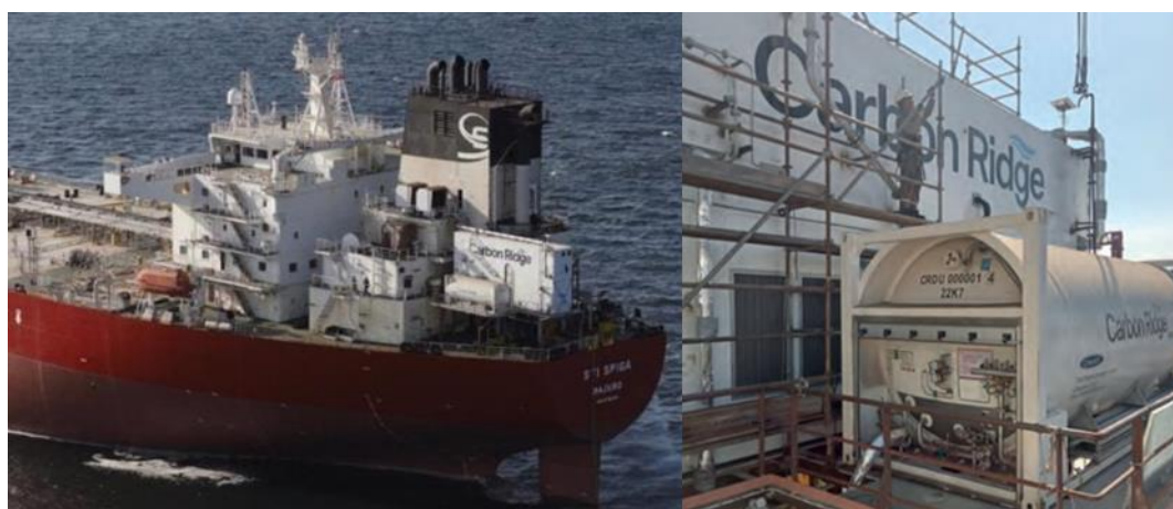
Figure 30. Carbon Ridge Installation on board STI Spiga
